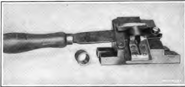
Fig. 11. Fixture for Holding Bushings when Milling Oil-groove
